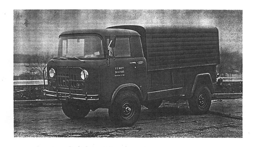
TRUCK, CARGO PICKUP, DIESEL ENGINE, 7000 GVW, 4 X 4 WILLYS MOTORS, INC., PILOT MODEL FC-170 WITH CERLIST DIESEL ENGINE FSN: 2320-889-2004
